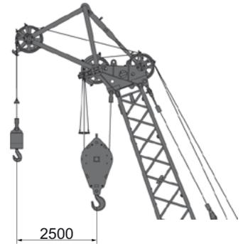
The optional auxiliary jib is designed for single strand operation up to max. 35 t. Conditions for lifting operations apply for rated loads.
